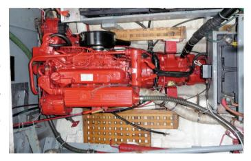
engine revs dropped suddenly from 2100 to 200. The cause of this was eventually found to be a blocked fuel filter. At that time I thought that this was due to dirt in the starboard fuel tank and a new filter was fitted and all resumed to normal once again. However over the intervening years the problem has persisted on and off.
